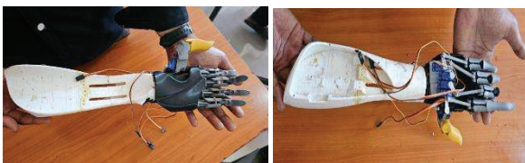
Fig: 5.1 Up side and Down side view of printed Arm with components assembled
