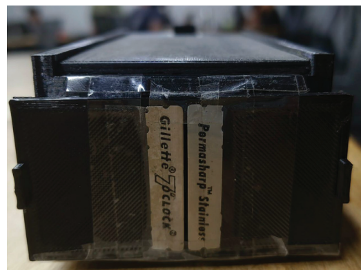
Fig 5 Slit of Spectrometer
